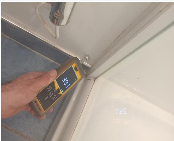
Moisture testing adjacent shower – dry range
