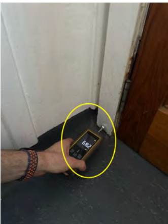
Slightly damp either side of rear door.
