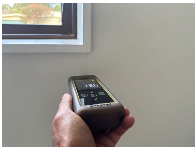
Moisture levels to the external walls scanned within the normal range at the time of inspection
