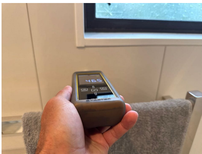
The moisture levels to the external walls were within the normal range
