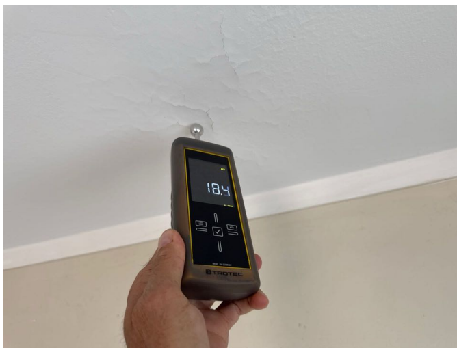
Deterioration to the ceiling lining above the oven does not appear to be moisture related. Possibly caused by a lack of extraction.
