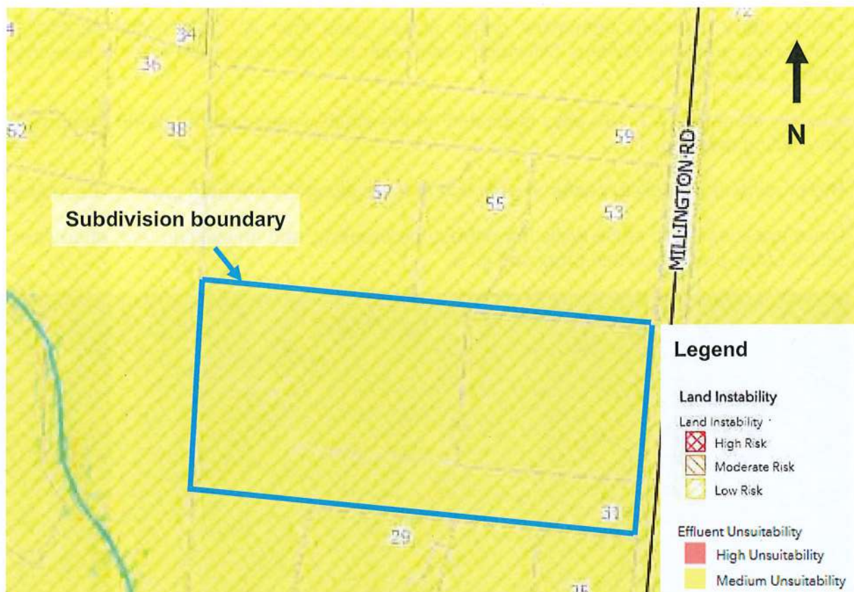
Figure B: Land instability and effluent unsuitability areas (source: WDC GIS Hazard Maps).
