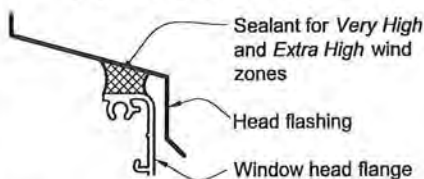
(c) METAL HEAD FLASHING SEALANT FOR VERY HIGH AND EXTRA HIGH WIND ZONES
