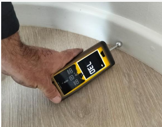
Elevated moisture readings taken on the exterior walls, being masonry walls the readings are not accurate/relevant.
