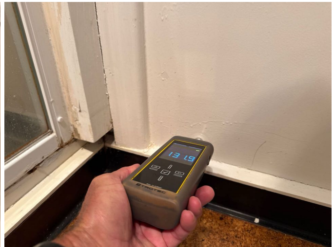
Elevated moisture readings to the external wall by the shower.
