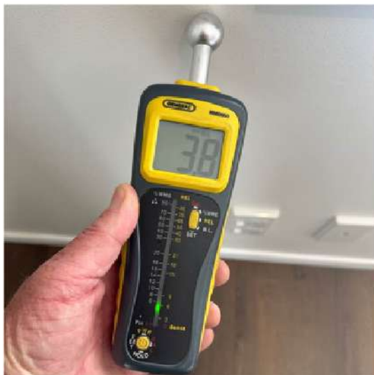
Low moisture reading, green = Good
