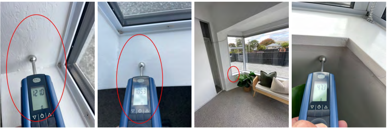
Elevated wet moisture readings noted in the SW bedroom window. Recent sealing has been done around the exterior of this window. It is recommended to retest for lower moisture levels here at a later date once this area has had time dry.
