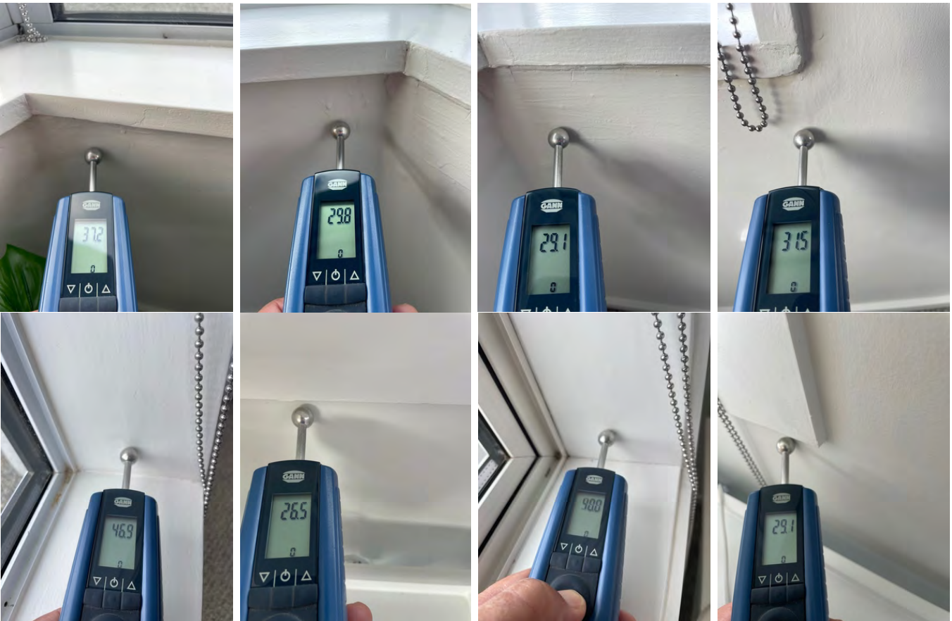
Elevated wet moisture readings noted in the SW bedroom window. Recent sealing has been done around the exterior of this window. It is recommended to retest for lower moisture levels here at a later date once this area has had time dry.
