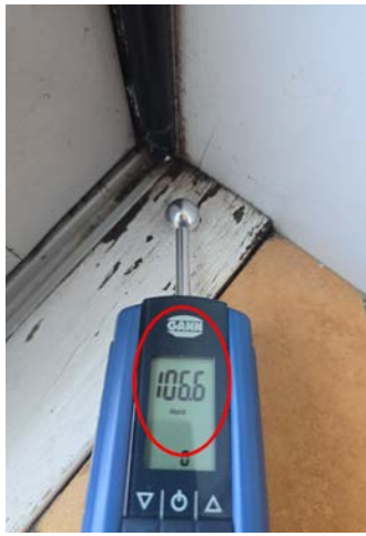
Elevated reading indicated on the external laundry door sill.
