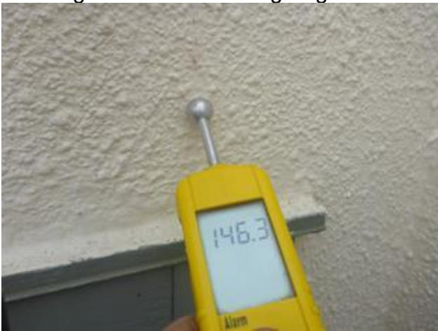
High moisture levels recorded to the cladding crack /front of the garage
