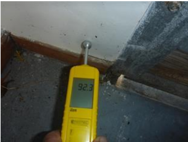
High moisture levels recorded ground level
