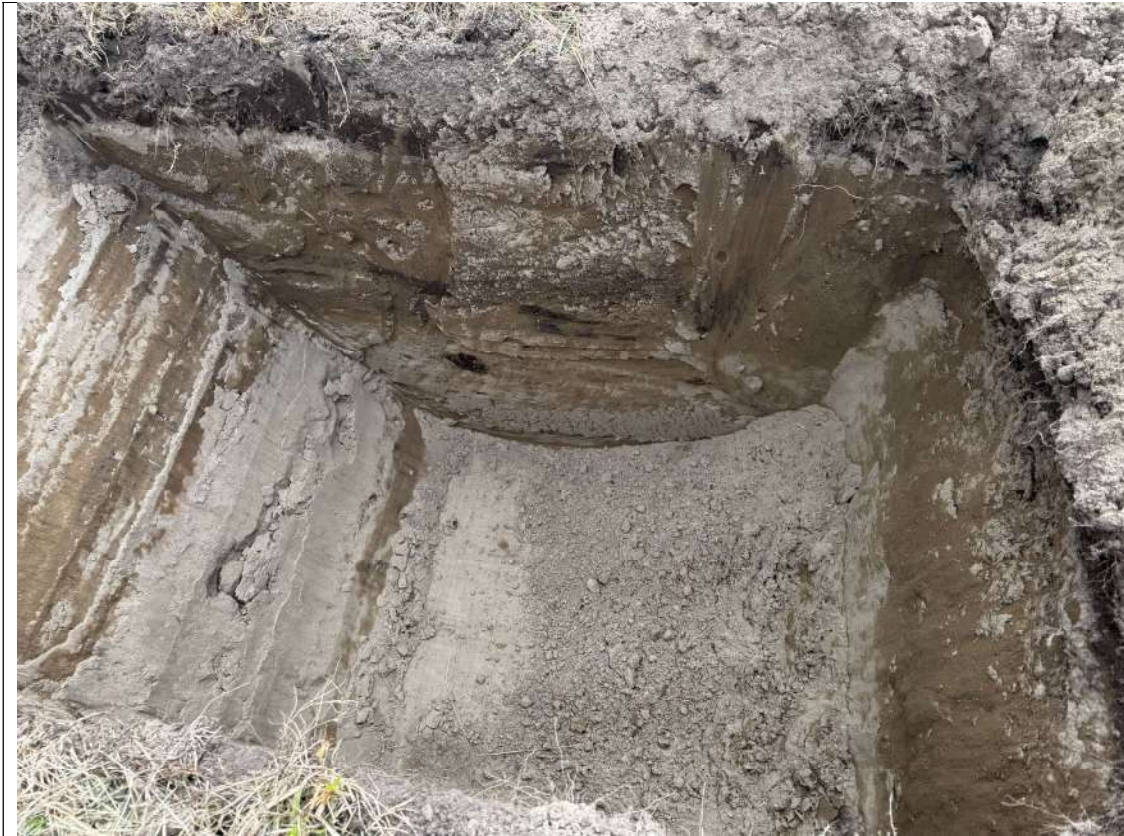
Figure 3: Image displaying excavated test pit. Image displays approximately 1.0-1.2m of FILL material. Small pockets of TOPSOIL are observed within the FILL material as displayed on the captured pit wall.
