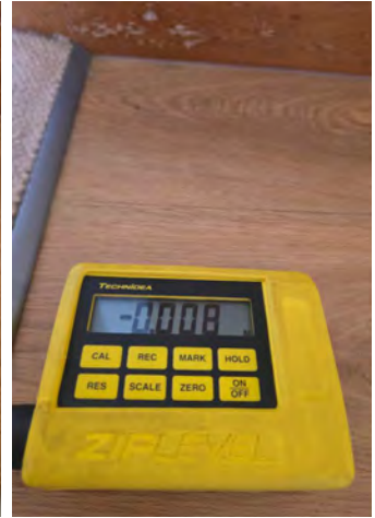
14mm stepdown to the composite board.
