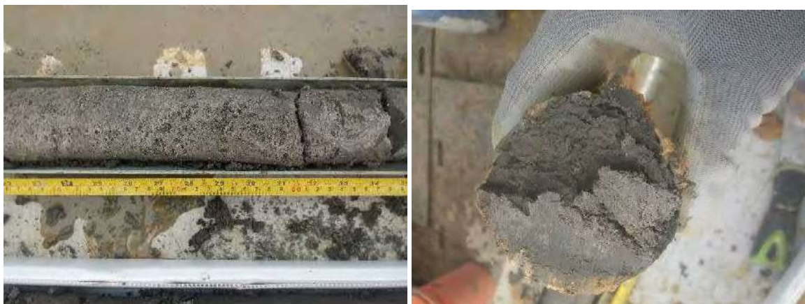
Figure 7-2: Typical Extremely Weak Mudstone Mélange within MBH20 – approx. 7 mBGL, with fabric (left) defect surface (right).
