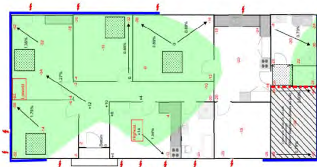
Figure 5 Precision floor plan with foundation crack locations indicated
