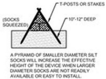
Pyramid installation staking
