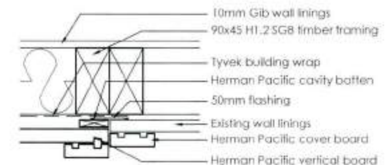
10 6 Cladding junction detail Scale 1:5 @ A3
