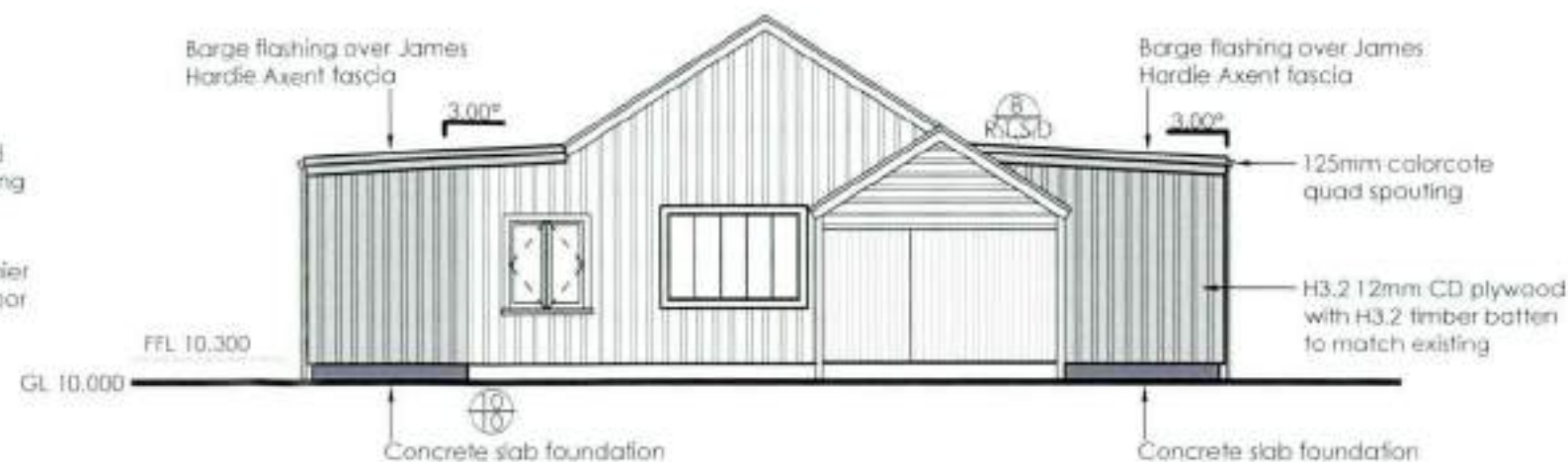
South West Elevation
