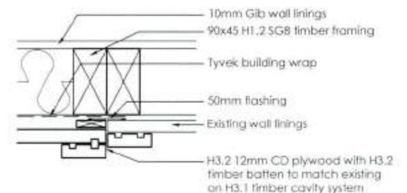
10 6 Cladding junction detail Scale 1:5 @ A3
