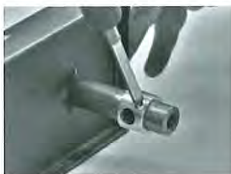
ULPG/Propane 11mm hole exposed
