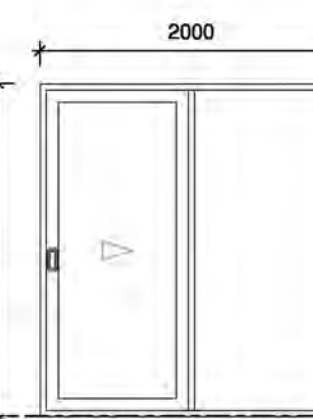
W9 SAFETY GLAZED SLIDING DOOR UNIT
