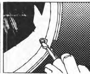
4. Tighten screws to draw fan firmly against ceiling. Then fit fly proofer and grille.
