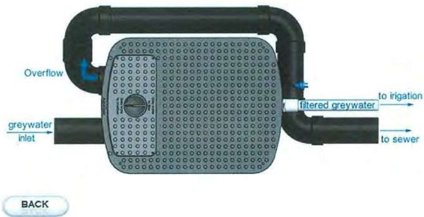
Figure: Top view of Aqua2use UG GWDD – example 4" connections
