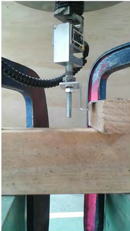
Load – pull-out test
