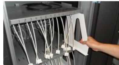
3. Loosen the thumb screws located on the front of the cable management channel above the shelf.
