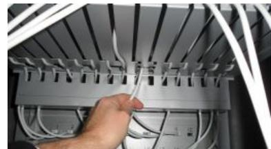
5. Unplug each cable from the USB connector in the back of the cart, and pull the cables through the cable channel and out of the cart.
