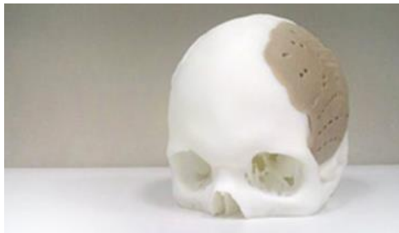
Figure 07 – a replacement plate for the human skull: printed using PEKK polymer.
