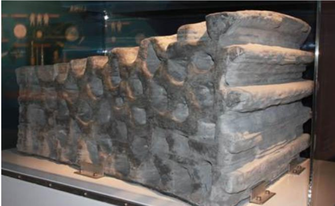
Figure 15 – The 1-ton (2,200 lb) test print of a wall from simulated lunar dirt.
