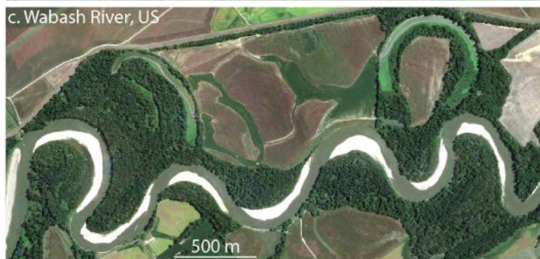
Figure 4.1: Examples of a. High-sinuosity meandering river characterized by abundance of vegetation along the river, a lack of bars, and neck-cutoffs (Rio Purus, Brazil); b. Low-sinuosity meandering river with low vegetation density and chute-cutoffs (Allier, France); c. Meandering river with bars forced by channel curvature (Wabash River, USA); d. Meander bend with free bars, including mid-channel bars (Rio Parnaíba, Brazil); e. Low-sinuosity river with free alternate bars (Cross River, Nigeria); f. Asymmetrical shape of the alternate bars with bar-tail limbs at the downstream (Indus River, Pakistan). Flow in all examples is from left to right. Source:
