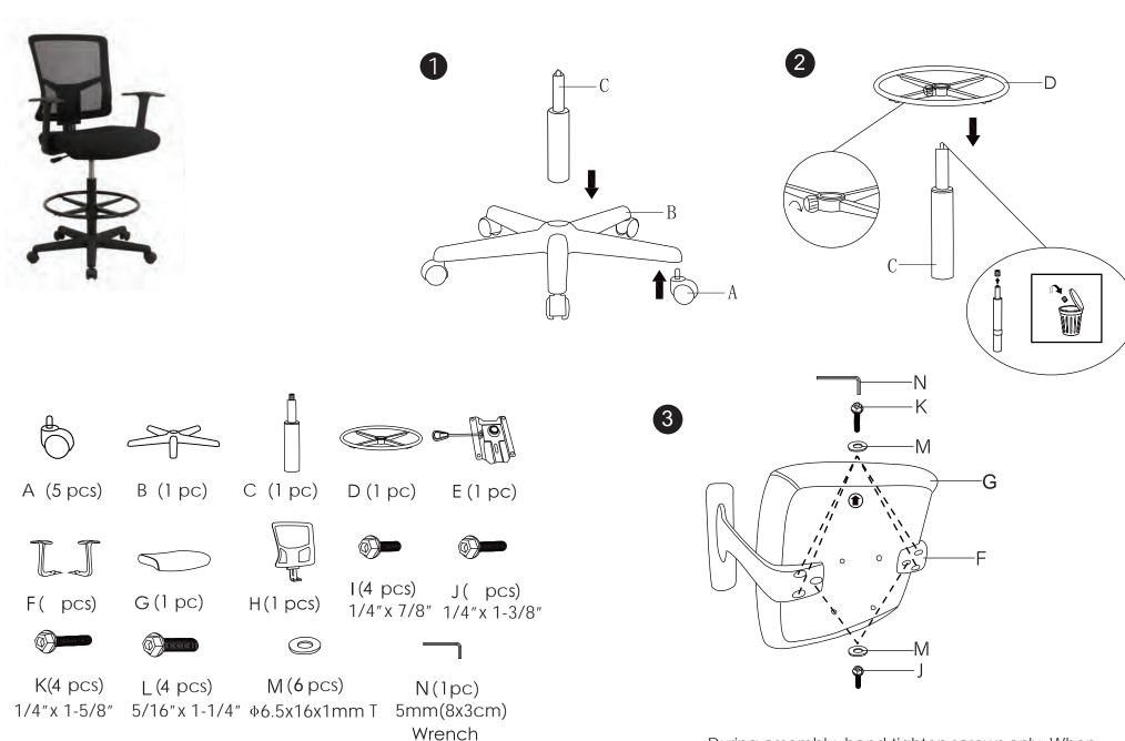
During assembly, hand tighten screws only. When the screws are in place, tighten completely.
