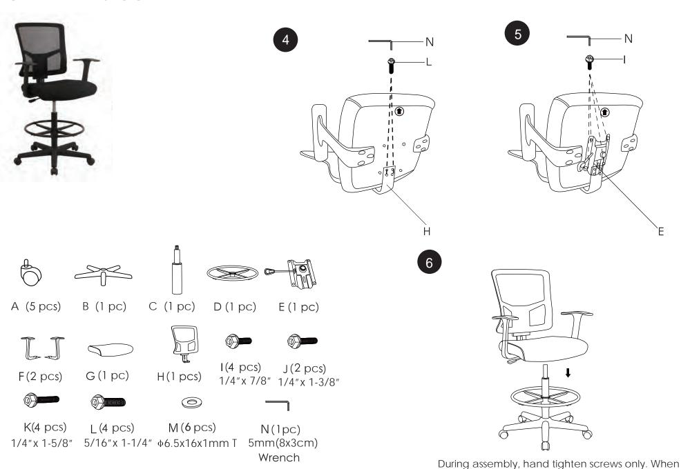
the screws are in place, tighten completely.
