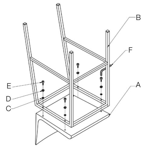
During assembly, hand tighten screws only. When all screws are in place, then tighten completely.
