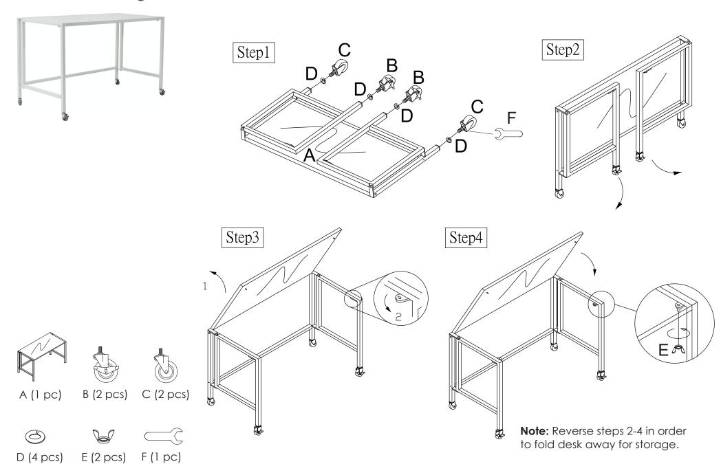
During assembly, hand tighten screws only. When the screws are in place, tighten completely.
