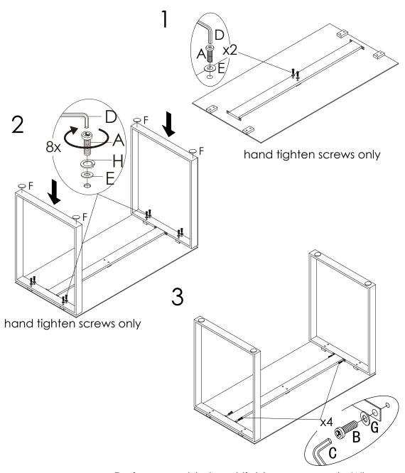
During assembly, hand tighten screws only. When all screws are in place, then tighten completely.
