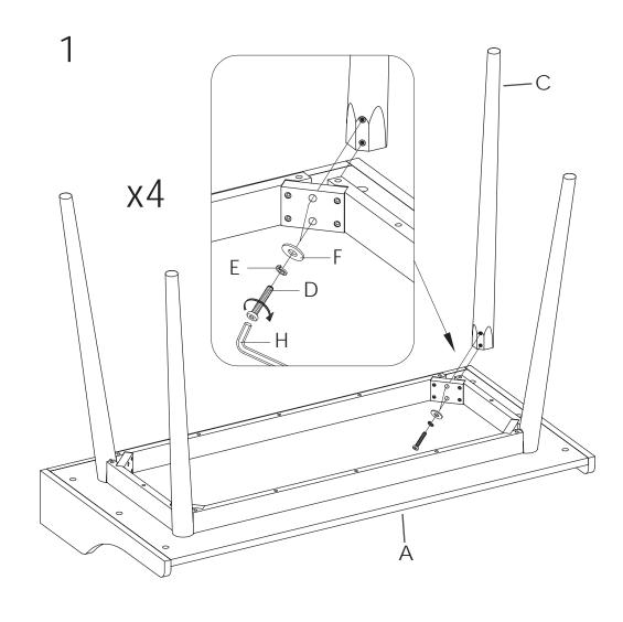
During assembly, hand tighten screws only. When the screws are in place, tighten completely.
