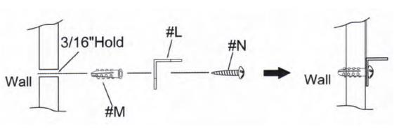
During assembly, hand tighten screws only. When the screws are in place, tighten completely.
