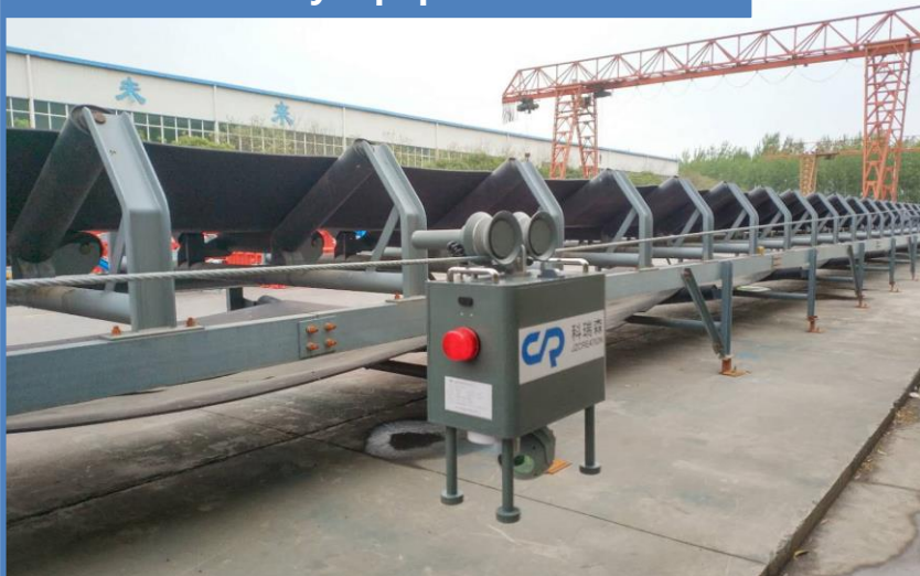
patrol inspection of bulk material to convey equipments
