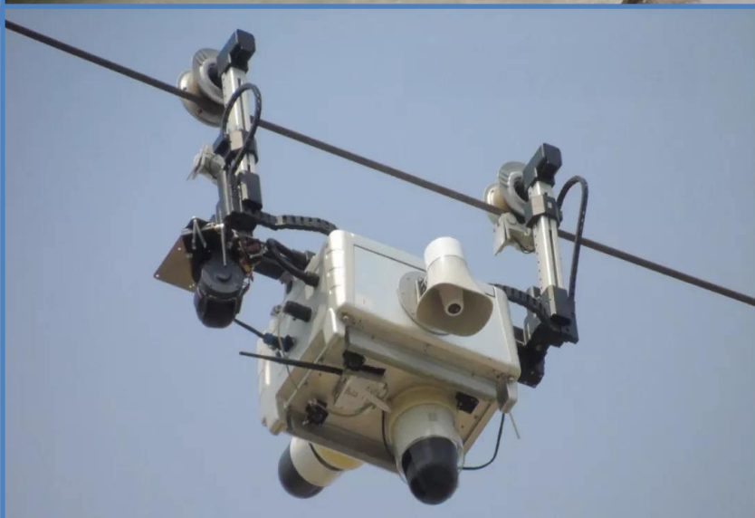
line inspection of overhead transmission
