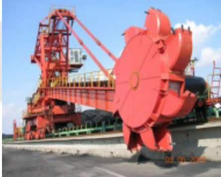
Bucket Wheel Stacker and Reclaimer
