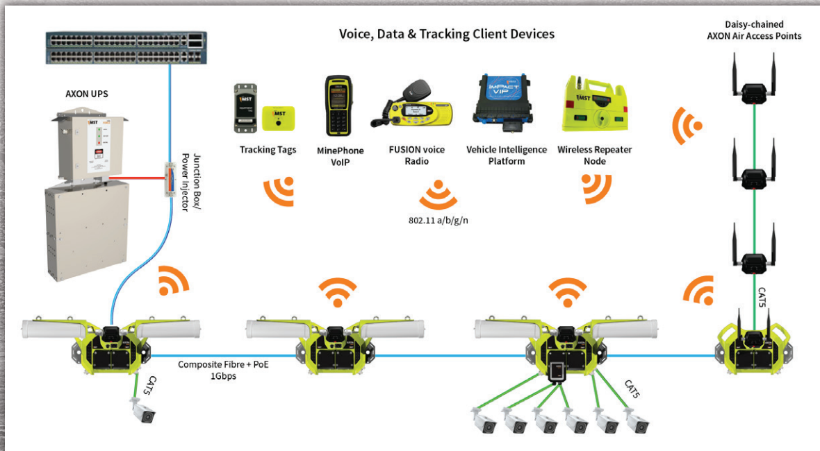
AXON infrastructure - A platform designed for supporting the many devices and applications required in the digital mine.
