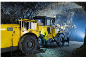
Bolt plan navigation, Rock reinforcement
