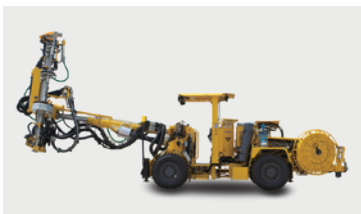
MBU (Medium bolting unit), Rock reinforcement
