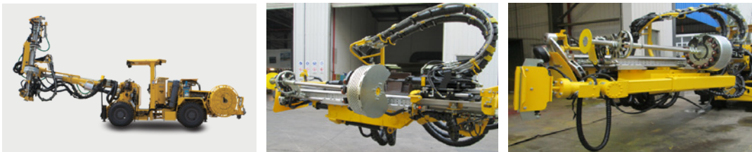
Screen handler, Rock reinforcement
