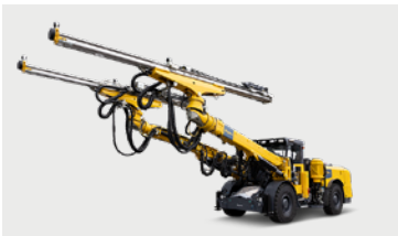
BUT 32, Face drilling
