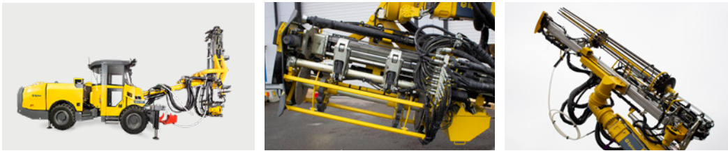
SBU (Small Bolting Unit), Rock Reinforcement
