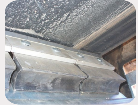
Razor-Back MDX with V-tip installed on this conveyor belt at a major copper ore mine.
