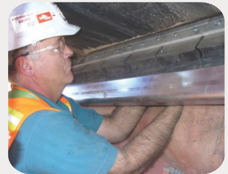
Razor-Back MDX is installed on this "super portable" stacker. It's easy to install and allows for simple removal of the cleaning cartridge.
