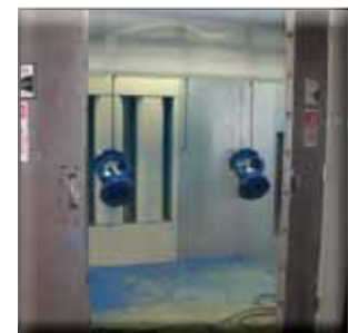
Automated Electrostatic Fusion Bonded Epoxy Process
