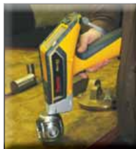
X-Ray Fluorescence Scanner provides Positive Material Identification (PMI)
