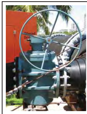
Cam-Centric® Plug Valve with worm gear actuator
