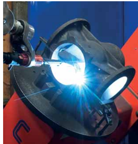
Figure 3. Robotic welding of nickel seat
