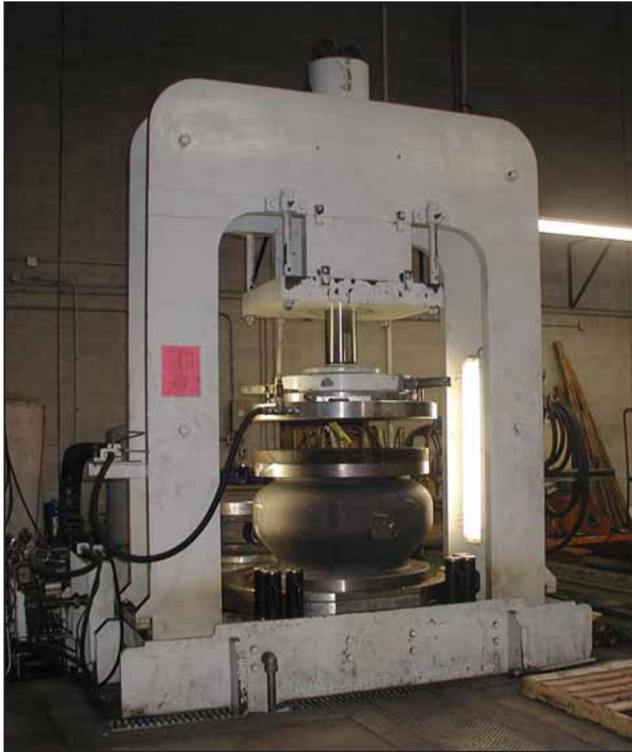
Silent Check Valve on a Test Stand
