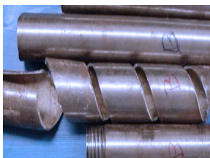
FATIGUE - SPIRAL DUE TO TORQUE
