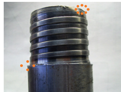
PIN SHOULDER AND PIN END FLARED DUE TO OVERLOAD
