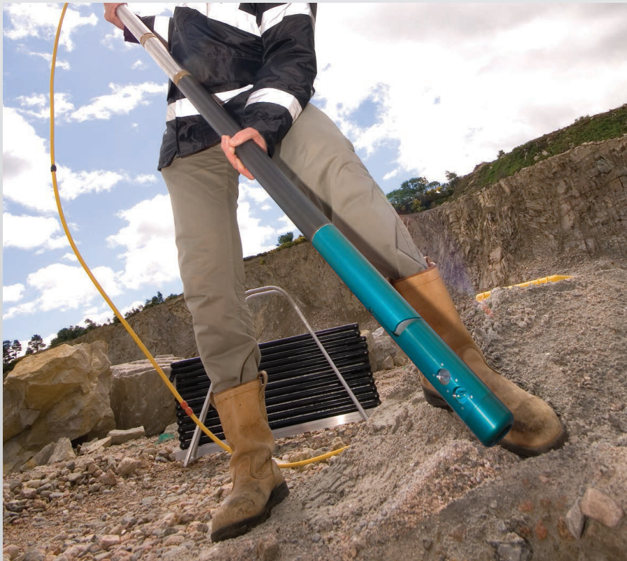
The nosecone camera provides a helpful view into the borehole during deployment.
