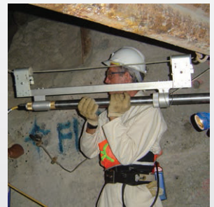
The C-ALS system deployed downhole to survey an inaccessible underground void.
