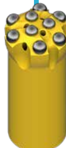
HARD ROCK Spherical buttons For tough conditions in hard and abrasive rock. Optimised face and body design and with large spherical buttons for long service life. Available with a short retract for straight holes in broken rock.
