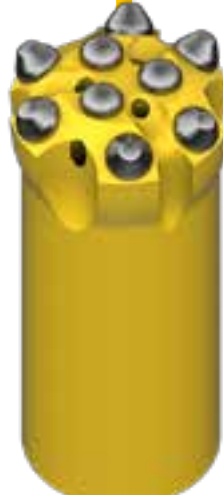
MEDIUM HARD ROCK Trubbnos buttons (gauge) and spherical buttons (centre) Ideal for abrasive, medium hard to hard rock. Larger Trubbnos buttons and flushing grooves give the ideal balance between service life and penetration rate. Available with a short retract for straight holes in broken rock.
