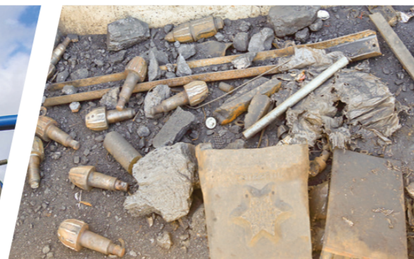
Tramp metal removed out of coal
