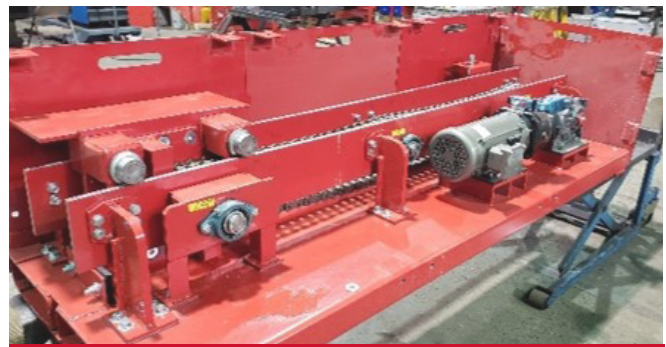
Drive Base Assembly for a Standard Duty Overhead Carriage Style Falling Stream Sampler
