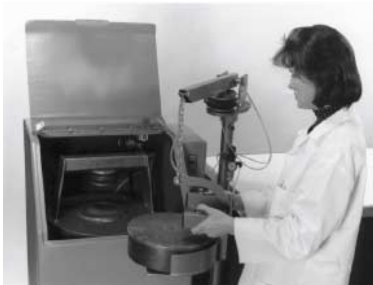
A Labtech Essa model B2000 bowl being carried “weightless” in the MILLMATE™ cradle. Note operators left thumb on one of the two push buttons that are used to raise and lower the cradle.
