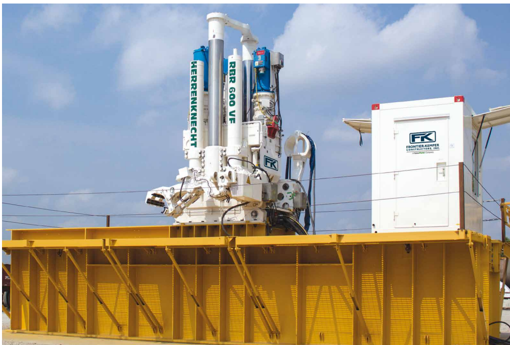
Fig. 7: RBR 600 VF mounted on a support frame for use over a presink
