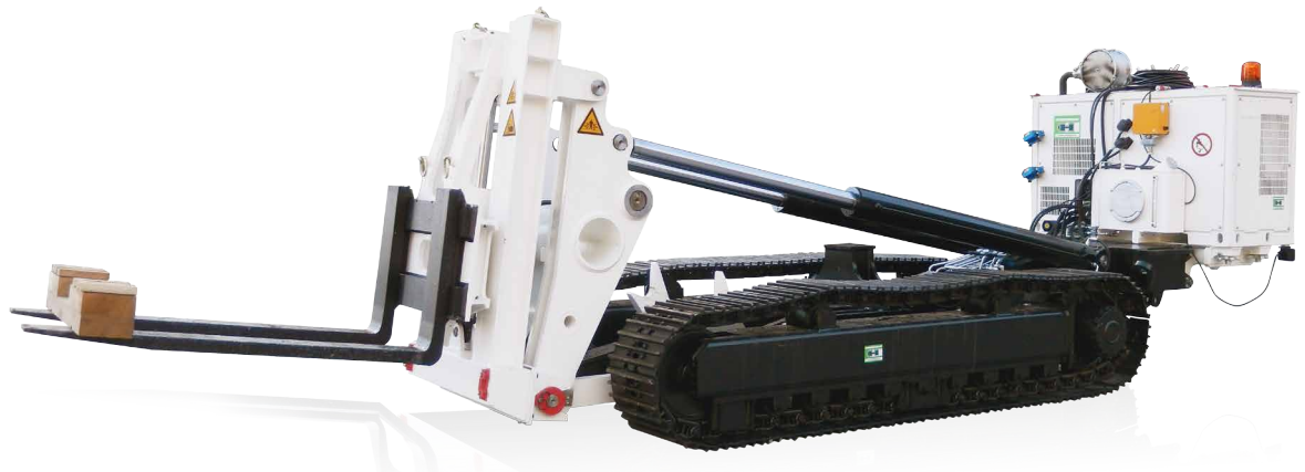
Fig. 5: Forklift equipment installed at the crawler unit
