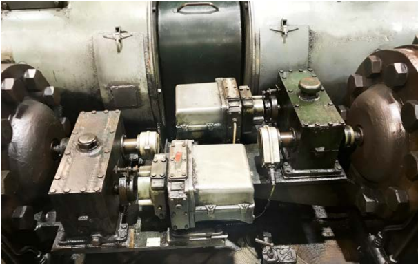
Antes: CAM Switch mecánico / Before: Mechanical cam limit switches
