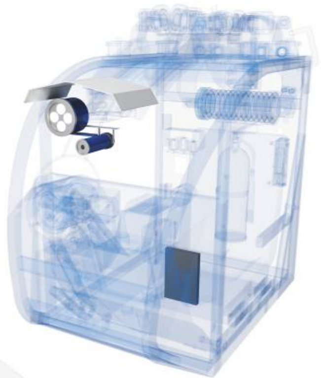
Monitoring system camera, projector and local monitor mounted in operator's cabin
