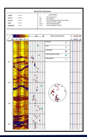
Reflection amplitude image, picked structures (tadpole presentation and stereographic projection, rose diagrams for the principal families of structures)
