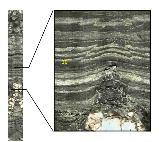
Optical image log example showing the level of detail that is possible to obtain (borehole dameter 96 mm - 3.8")
