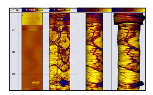
Acoustic imagery example showing a "virtual core" created using the travel time and amplitude images.
