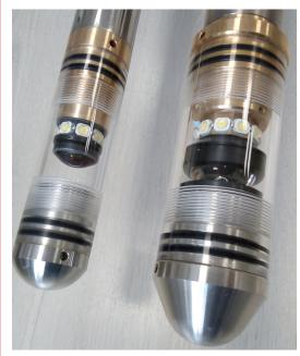
A precision wide angle lens and a CMOS camera assembly permit the OPTV38 and OPTV52 probes to capture a high- definition video image of the borehole wall in a variety of horizontal and vertical resolutions. The resulting image data is digitised in the probe and combined with orientation sensor parameters for transmission to the surface.
