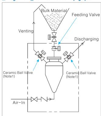
Note1: Pneumatic Ceramic Double Disc Valve is optional This is a typical pneumatic conveying unit, and other similar systems are also applicable.
