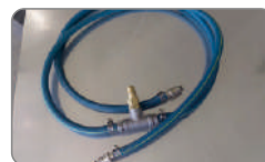
Cooling System Pipe Blue cold water inlet
